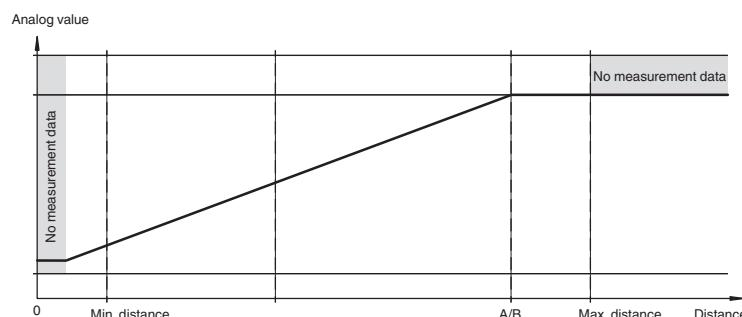
**Rising slope (A < B)**
